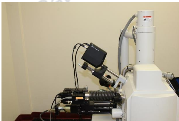
Figure 4 Working arrangement of EDAX (Energy dispersive analysis of X-rays)
